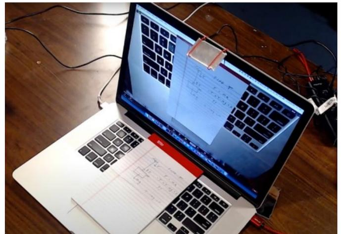
An issue is how to write on top of the keyboard? A simplest solution is to create a small table that can lay on top of the keyboard as seen below. The table just needs to be large enough to cover the keyboard and have room for “legs” in each corner. An example of legs can be left over from packaging, dowel rods, small pieces of
